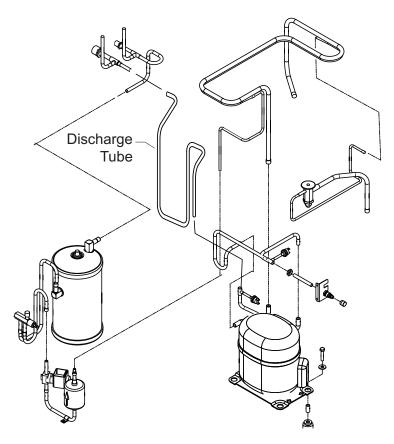
Recommendation: When changing a compressor on a unit built before the design change, order a new discharge tube and change it as well.
